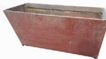
Hot elevator bucket
